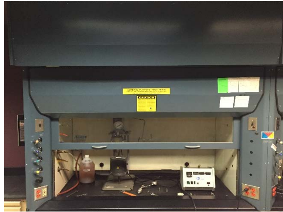
Auxiliary air hood on GT's campus
